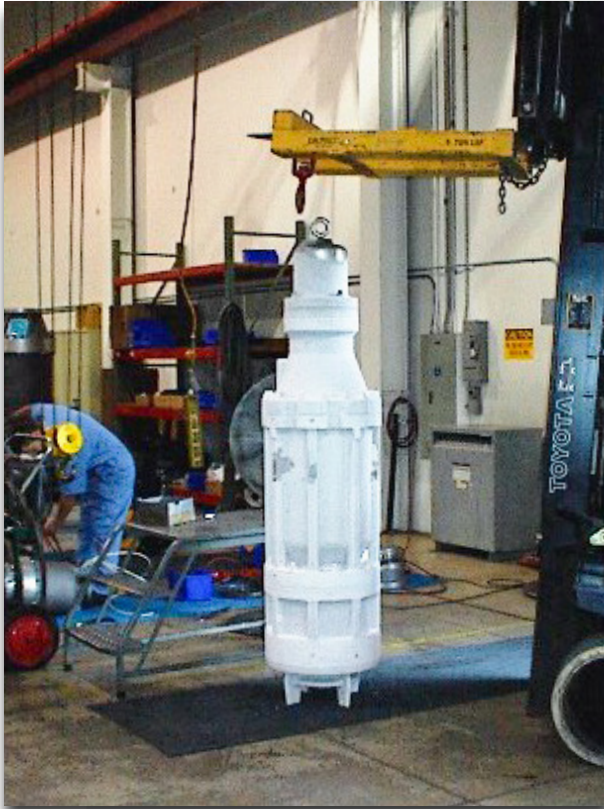
EMERGENCY PUMP AFTER TESTING
